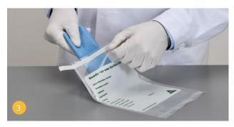
Put the swab into the sterile Twirl-Tie  $^{\text{TM}}$  bag and label bag with sample details. Always switch gloves between sampling sites.
