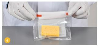
Close the Twirl-Tie  $^{\text{TM}}$  bag with the wires attached and label it. No gloves needed.
