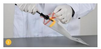
Release sponge from the quick release handle into the Twirl-Tie $^{TM}$  bag provided, by pulling the clip back.
