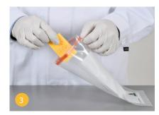
Put sponge into the sterile sample bag (or back into the vial) and label bag with sample details. Always switch gloves between sampling sites.
